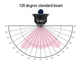
With regards to light distribution SM01 have opted for a wide beam120 degrees output. In this way you can easily obtain a perfect flat light level over bars, what makes the system also suitable for lower crop light levels.
